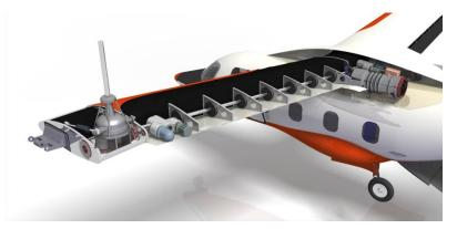
The *HeliX* was designed with *turboshaft engines*, based on the 2007 AHS Student Design Competition "rubber" engine model, for increased reliability and minimized cost.
