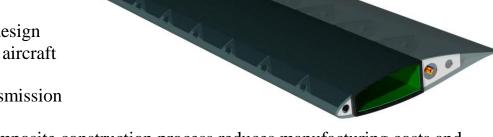
✓ Out-of-autoclave composite construction process reduces manufacturing costs and permits high quality assurance
