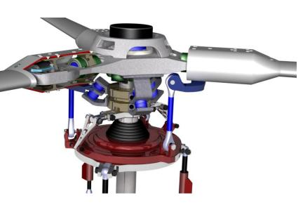
blade flapping. This in turn reduces in-plane bending moments from lead-lag.
